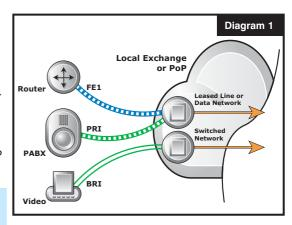
The Carrier can deliver a single PRI ISDN service to site with Liberator presenting a flexible combination of services to the client that can easily be modified.
